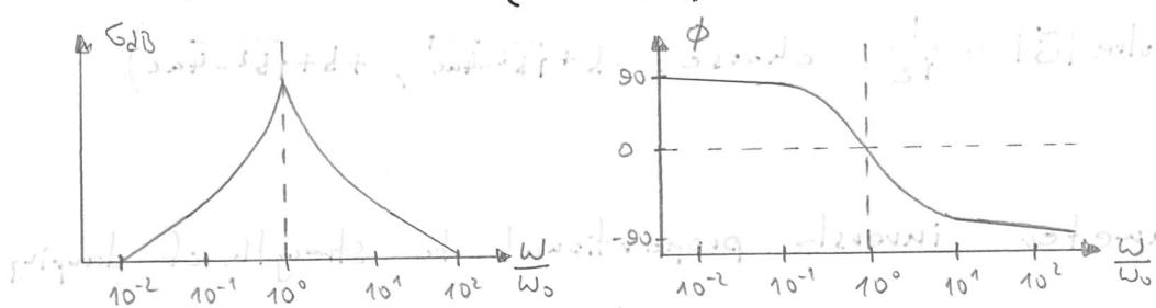
↪ used in analogue radio tuner. air capacitor is adjusted to change  $\omega_0$
