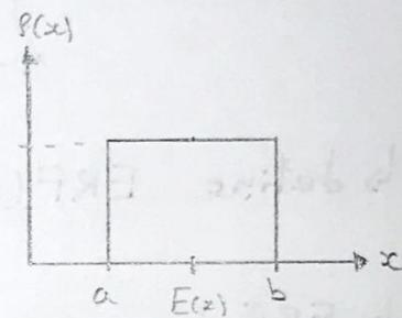
$$E(x) = \frac{a+b}{2} \quad V(x) = \frac{(b-a)^2}{12} \quad \text{so} \quad \sigma(x) = \frac{b-a}{\sqrt{12}}$$
